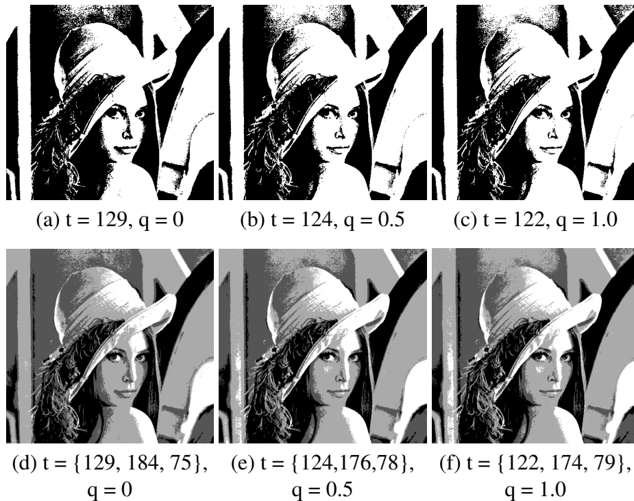
Figure 5 – The segmentation of lenna image for q = \{0, 0.5, 1.0\} . The first row presents the simple non-extensive algorithm and second row presents the corresponding recursive version. t stands for the found threshold value.
